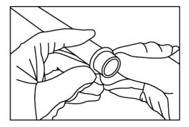
5. Place the quartz sleeve inside the stainless steel chamber.
