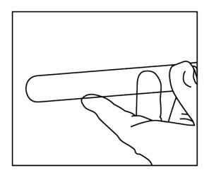
4. Install the O-ring on the open side of the quartz sleeve (0.47 inches from the edge).
