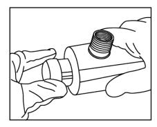
7. Connect the 4-pin UV emitter bulb to the electronic ballast.
