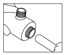
6. Screw on the stainless steel chamber cap. Avoid overtightening the cap to avoid damaging the O-ring or quartz sleeve.
