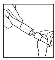
8. Carefully insert the UV emitting bulb into the quartz sleeve through the open cover.
